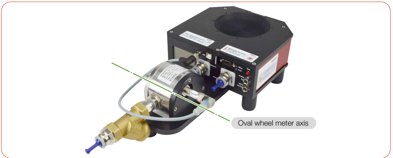
Fig. 6.1: Position of the oval wheel meter axis (using the CPM F-10 as example)
